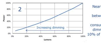
Near proportional relationship between dimming and power consumption when dimming down to 10% of max. power. More energy efficient than HPS.
