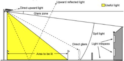
Upward reflected light cannot be controlled by the lighting engineer if they have no control over the surface. However, it should be noted that reflectivity coefficients vary greatly depending on the surface.
